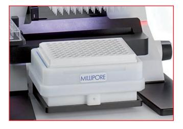
In addition to the different pipetting heads for different volume ranges, there are various accessories available to support additional laboratory tasks. Multiple clean-up methods can be automated very easily through the use of a vacuum chamber. Also an orbital shaker can be used in addition to the 2-positions for microplates and reservoirs. Through the use of heating or cooling solutions, temperature dependant applications are easily realizable.
